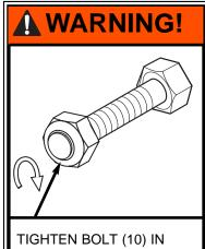
TIGHTEN BOLT (10) IN LOCK NUT (5) UNTIL FLUSH (EVEN) WITH LOCK NUT'S OUTER EDGE.
